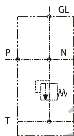
③ Top Inlet Port with DPRV & Side Gauge Port
